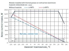
Fig.6.1. Temperature derating MAA1500
