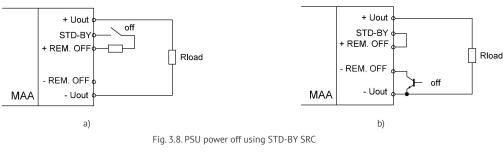
Ha Fig.3.8b shows the module that will shut down when closing power off to -Vout.
