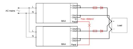
Fig.5.2. Redundancy connection
