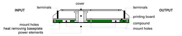
Output pins or terminals are grouped on opposite sides of the case: input ones are located on one side, while the output ones are on the opposite. Inputs and outputs are isolated from each other and from the housing, isolation voltage is specified in a datasheet for each PSU model. Multi-channel modules also have their output channels isolated from each other, allowing to connect them in series or to form bipolar voltage.
