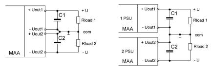
Figure 5.4. Examples of obtaining bipolar output voltage
