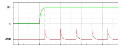
Fig.4.1. PSU's operation in short-circuit mode
