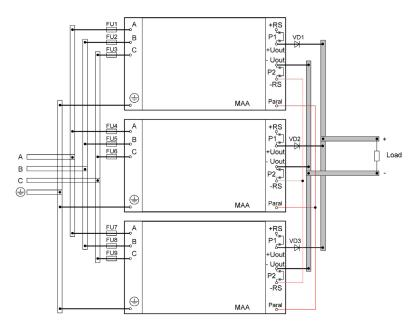
Fig.5.1. Parallel connection
