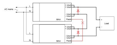
Fig. 5.3. Example of reaching high voltages by summing up the voltages of output channels.
