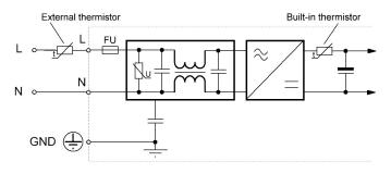
Fig. 5.7. Passive limiting of in-rush current using external thermistor.
