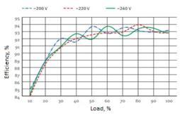
Fig. 6.3. MAA75C24XX efficiency VS output power
