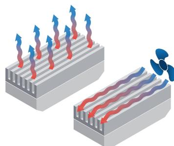
Material for the heatsink can be chosen either an ordinary metal (less often ceramic) plate (including the wall of the case or cabinet), and what is meant by the word “radiator” is usually a plate with a ribbed or needle-shaped surface. Its task is to increase the contact area with the cooling agent, which can be both any gas (air, hydrogen, helium) and liquid (water, glycol, oil).
