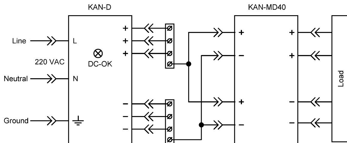
Application example KAN-MD40+KAN-D in parallel operation.
