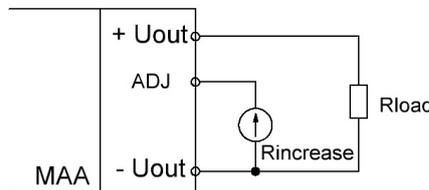
Fig. 3.10. Connecting an external voltage source to adjust the output voltage of the power supply unit.
