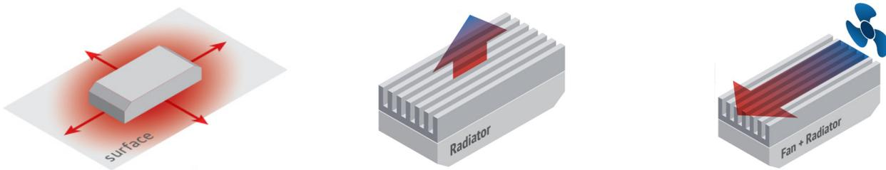
Fig.6.2. Types of conductive cooling.
