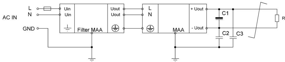
Fig.5.13. Recommended circuit for improved EMC and reduced output ripple.
