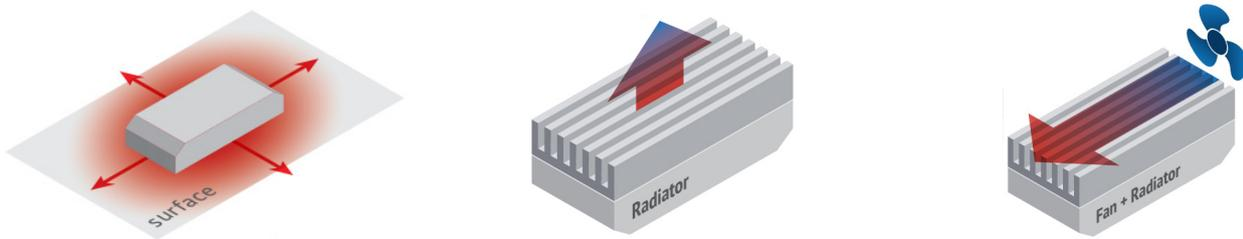
Fig.6.2. Types of conductive cooling.
