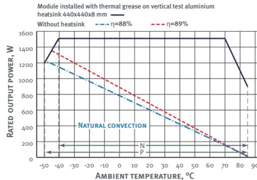
Fig.6.1. Temperature derating MAA1500
