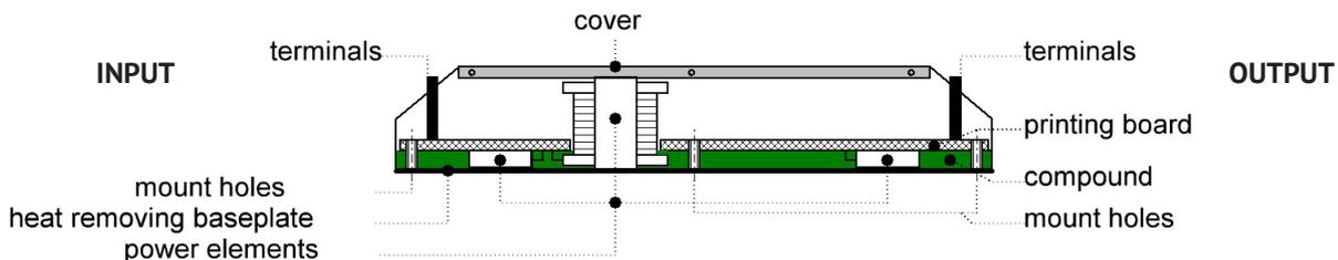
Output pins or terminals are grouped on opposite sides of the case: input ones are located on one side, while the output ones are on the opposite. Inputs and outputs are isolated from each other and from the housing, isolation voltage is specified in a datasheet for each PSU model. Multi-channel modules also have their output channels isolated from each other, allowing to connect them in series or to form bipolar voltage.
