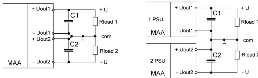
Figure 5.4. Examples of obtaining bipolar output voltage
