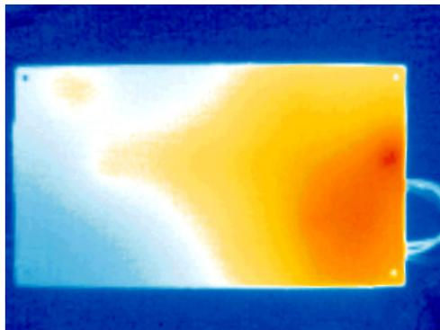
Fig. 6.4. Heat map of MAA1500-1S48SGN without heat sink, the hottest point is +50°C.
