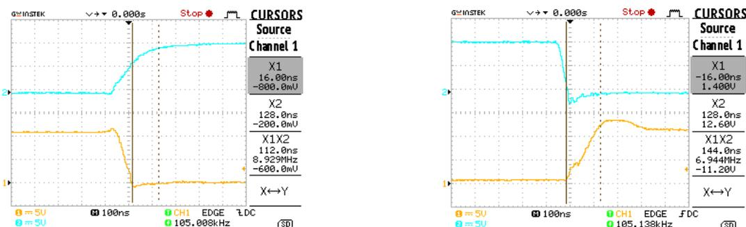
Fig. 3.7. Timing diagrams of MAA1500-1S24SGN power on and off by DC voltage at Remote OFF/ON pin are shown in the oscillogram.
