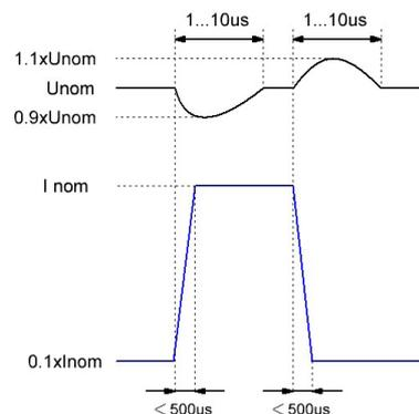
Fig. 5.5. Transient deviation of output voltage with pulse load (a - output voltage, b - load current).
