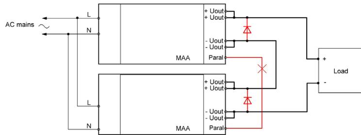
Fig. 5.3. Example of reaching high voltages by summing up the voltages of output channels.
