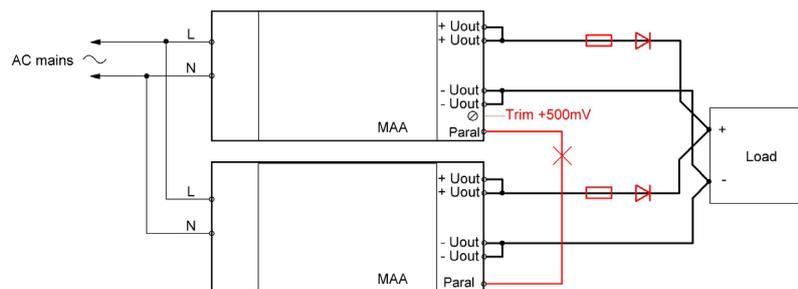
Fig.5.2. Redundancy connection
