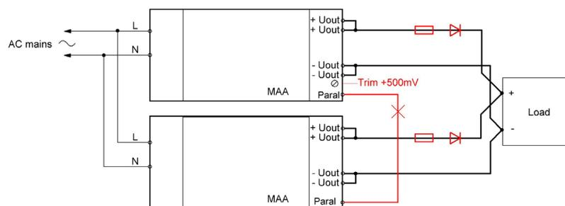
Fig.5.2. Redundancy connection
