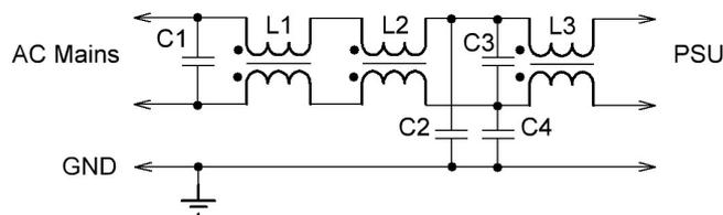
Fig. 5.14. Circuit for external EMI filters connected to the input of a PSU
