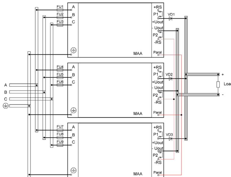
Fig.5.1. Parallel connection
