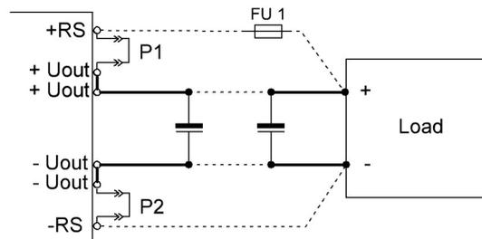
Fig.3.4. Remote load operation
