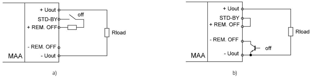
Fig. 3.8. PSU power off using STD-BY SRC
