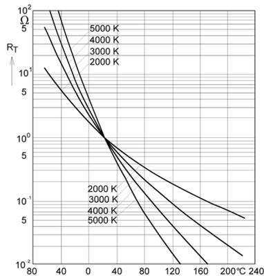
NTC-thermistor resistance VS temperature
