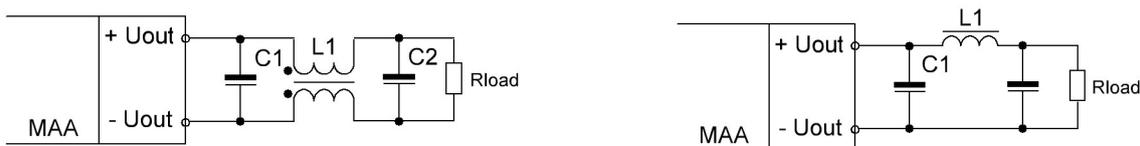
Fig.5.10. Examples of connecting output filters
