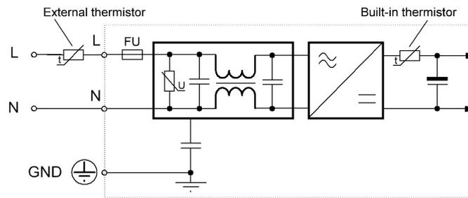
Fig. 5.7. Passive limiting of in-rush current using external thermistor..
