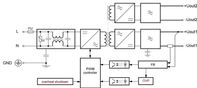
Fig.3.1. Block diagram of a dual-channel PSU MAA30-2XXX
