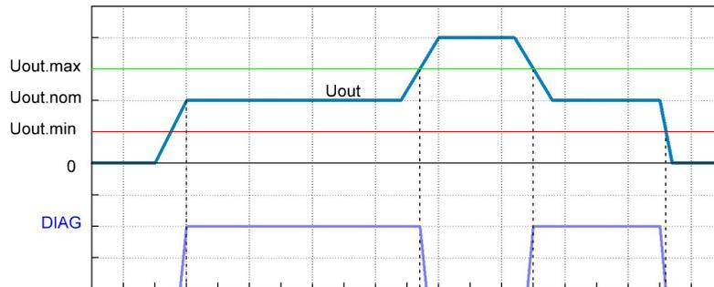
Fig. 3.3 Timing diagram of DIAG output operation.
