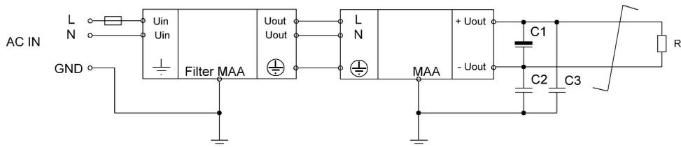
Fig.5.13. Recommended circuit for improved EMC and reduced output ripple.
