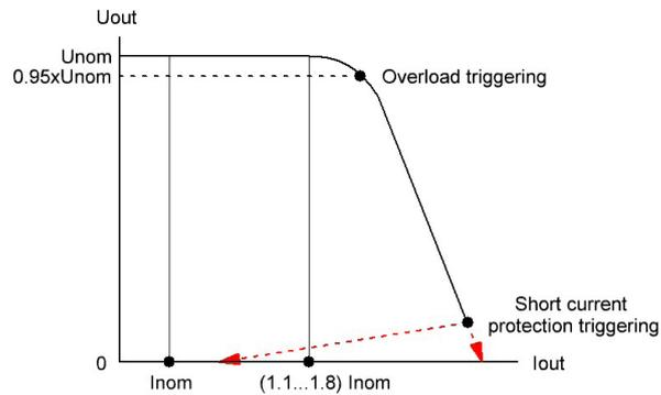
Fig.4.2. Output characteristic
