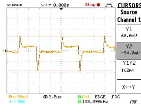
Fig.5.9. Output ripple
