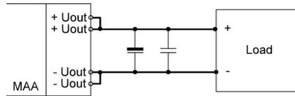
Fig 5.6. Connection of output capacitors
