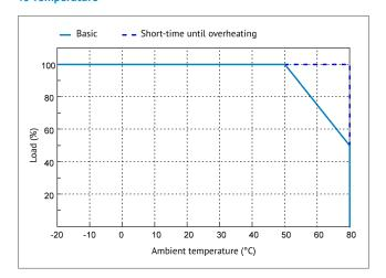
Diagrams show results of testing KWadr5000C300, vertical axis relates to the Load (%).
