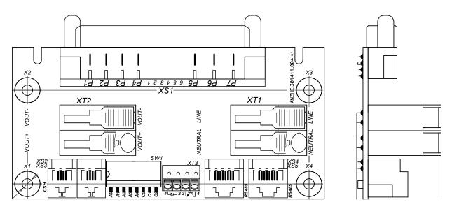
For separate use of KWadr5000 unit it is necessary to use KWadr5000 connection board. If KWadr5000 unit is used with KAP-series the KWadr5000 connection board is not necessary. Dimensions of KWadr5000 connection board see at page 10.
